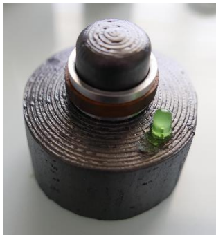
Figure 4: Induction charging bay for MemoRing
